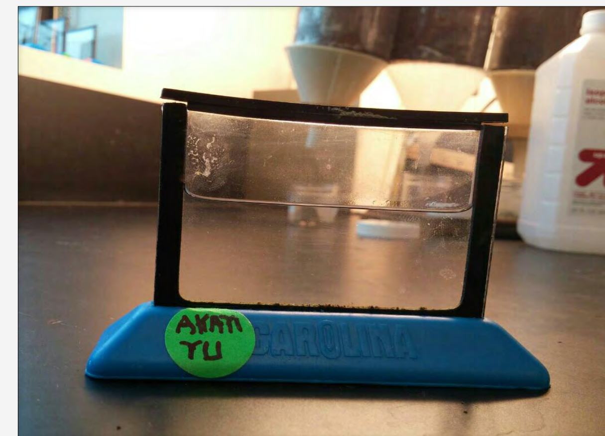
Figure 2. The microaquarium (Carolina Biological) is 75 × 50 × 4-mm and holds about 5 ml.
